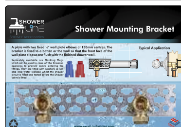
Shower Valve Mounting Bracket
